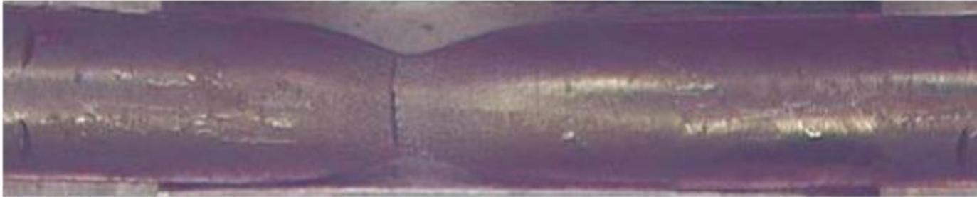
Specimen EL4 – Tested at 49°C
