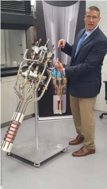
Marc Gibson, NASA Glenn's Kilopower Lead Engineer, explains the operation of the KRUSTY Kilopower prototype design to members of the media at NASA Glenn's Sterling Research Lab in Cleveland, Ohio. Photo Credit: Michael Cole / Spaceflight Insider
