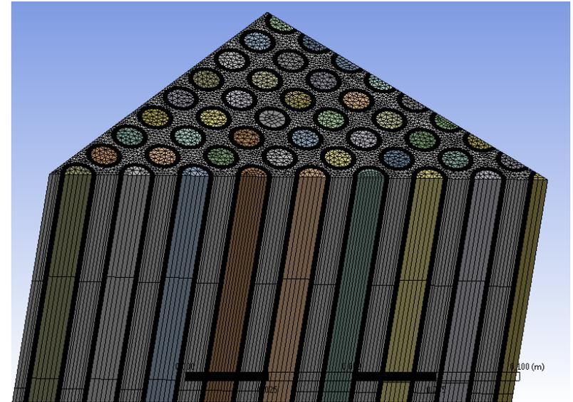
Figure 4 – Isometric View of Domain Discretization
