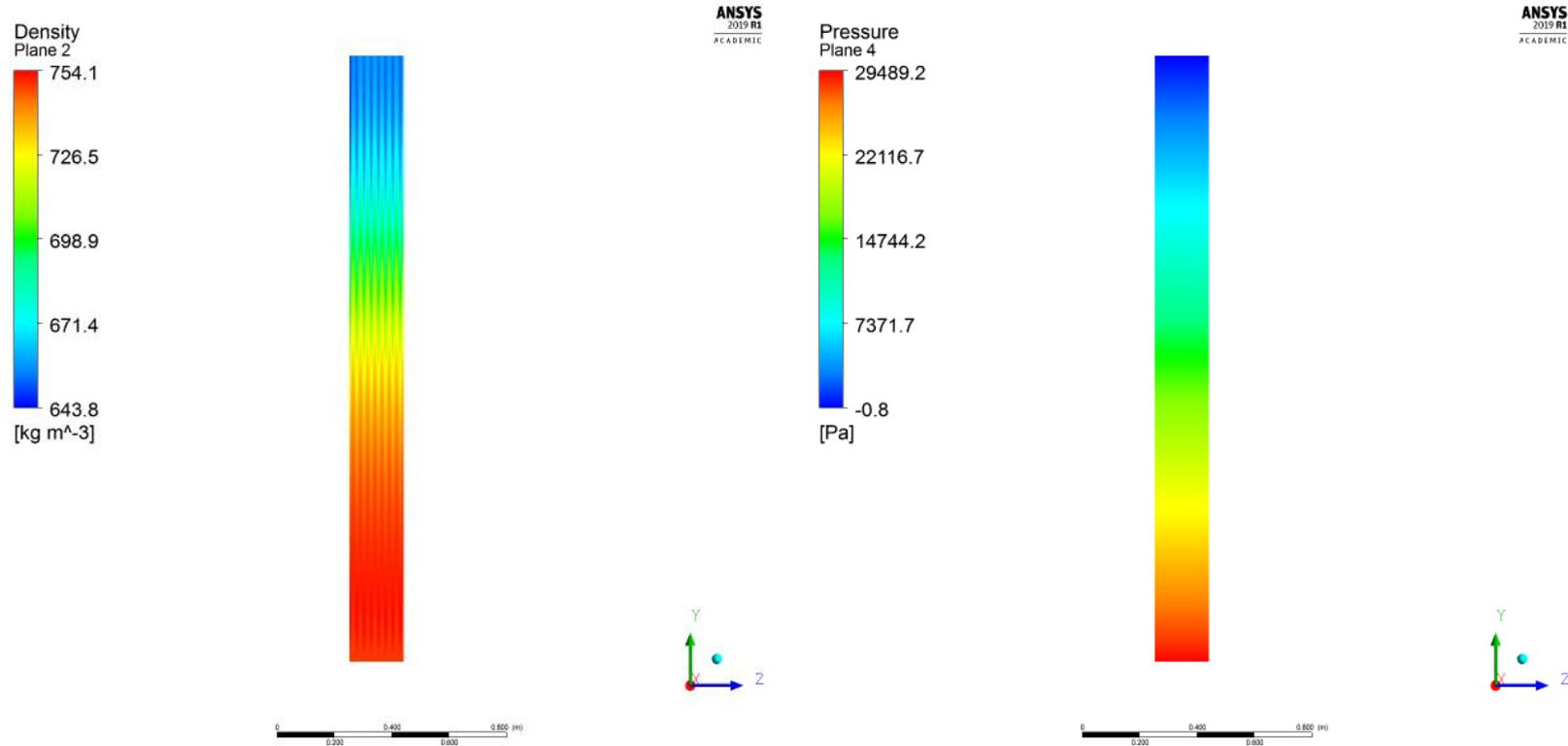
Figure 8 – Axial Distribution of Coolant Density and the Pressure Drop Along the Fuel Assembly
