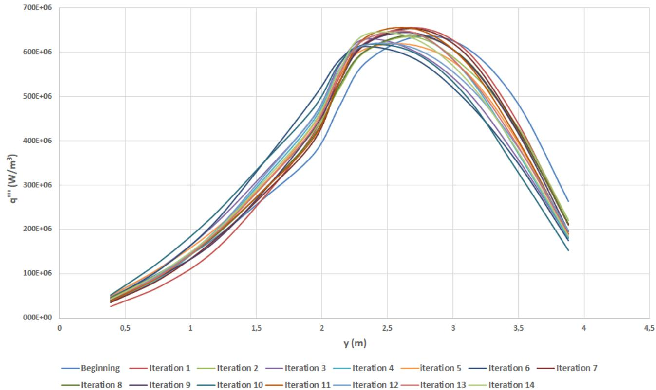
Figure 5 – Iterative Study of the Axial Distribution of Power Density.
