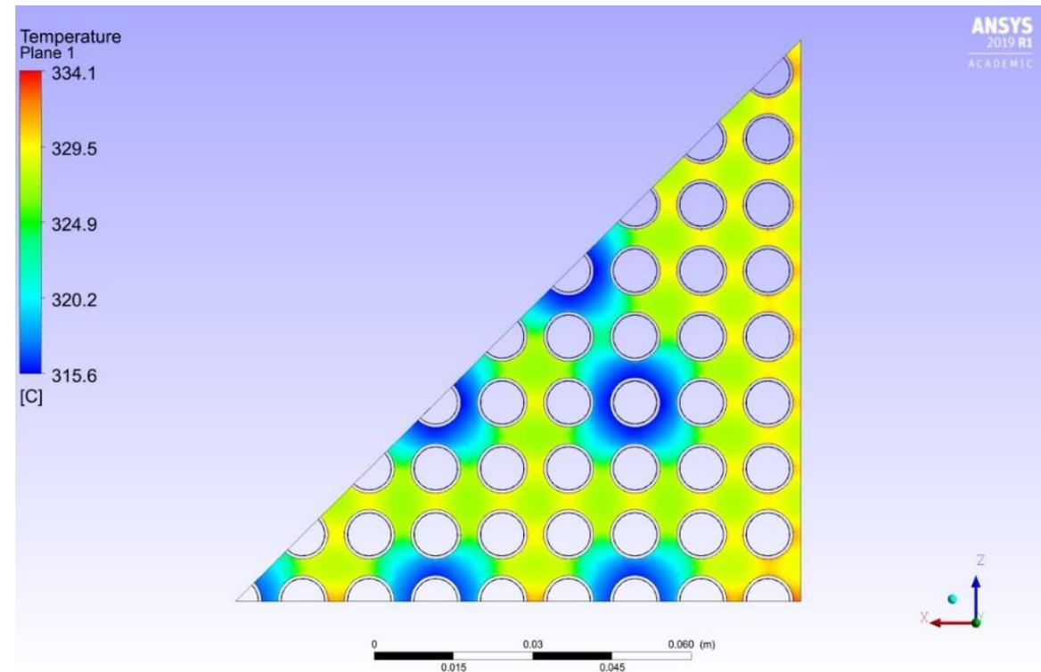
Figure 7 – Coolant Temperature Field at the Fuel Assembly Outlet
