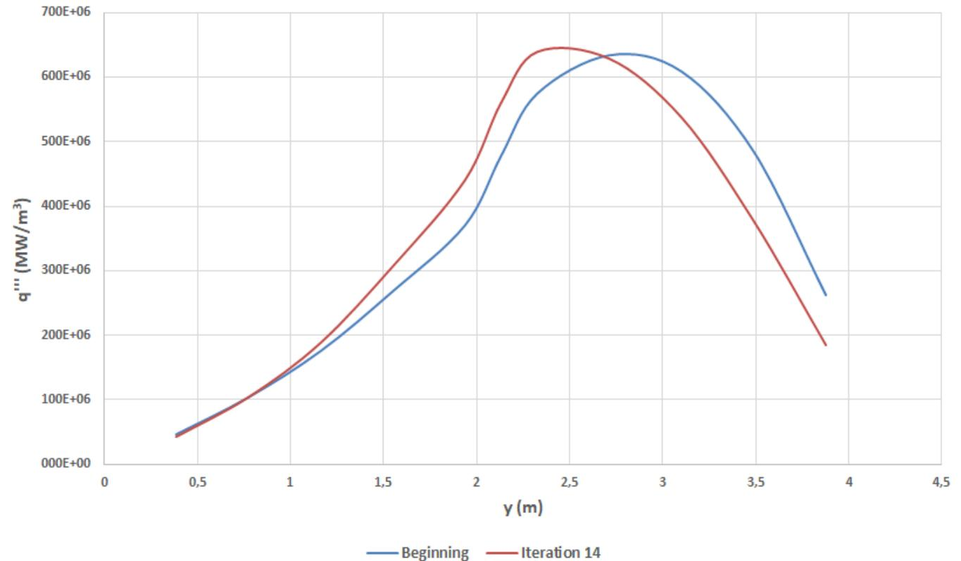
Figure 6 – Comparison of the Axial Distribution from the Power Density at Initial and Final States of the Iterative Process.
