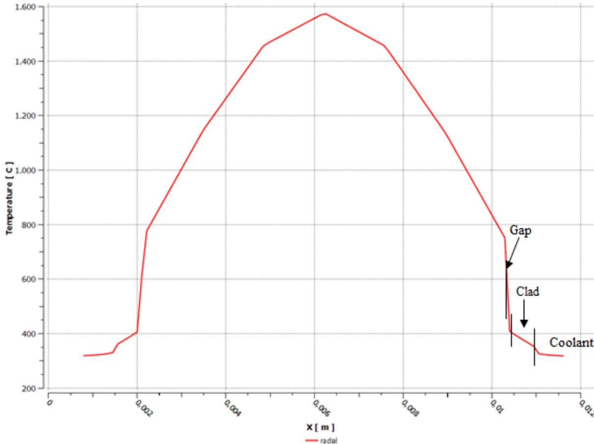
The maximum temperature reached in the cladding was 410°C;
