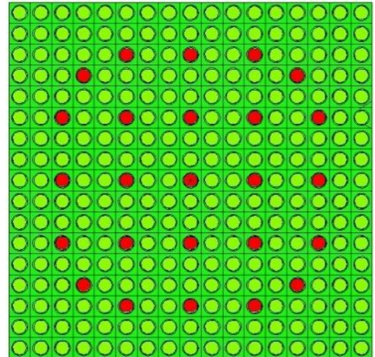
Figure 2 – Description of the Fuel Assembly Used to the Neutronic and Thermohydraulic Calculations.
