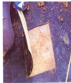
Studies on ageing of the bituminous membrane (Centre de la Manche)
