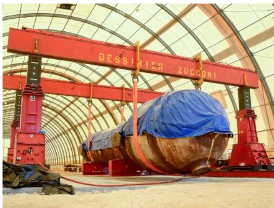
Decontaminated steam generator (VLL)
