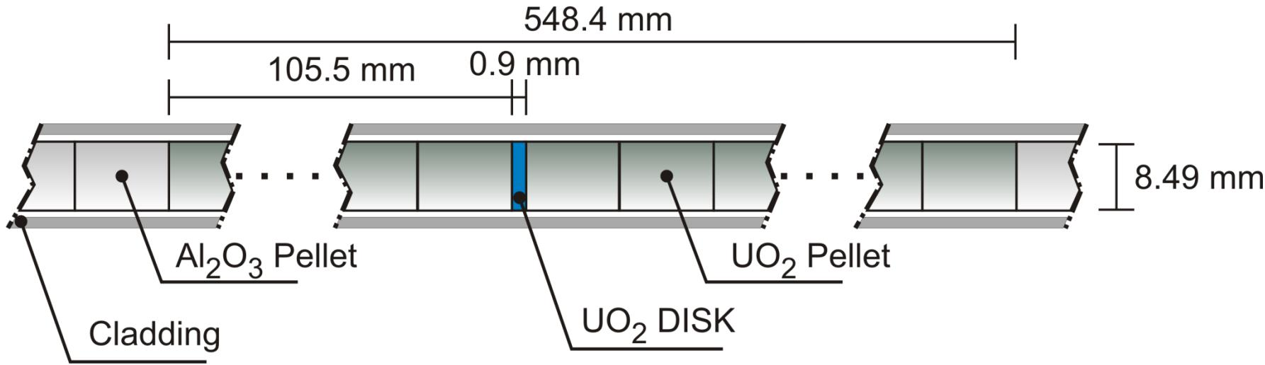
**The UO<sub>2</sub> disk was obtained cutting of the IPEN/MB-01 UO<sub>2</sub> pellets by a sharp tool. The Uncertainty in the UO<sub>2</sub> disk thickness was less than 1%.**
