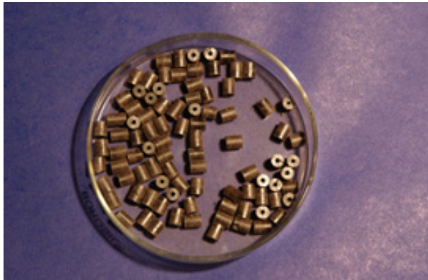
FIG. 4. Annular MOX pellet fabricated for the PFBR.
