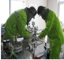
FIG. 1. Trainees dismantling the pipe of a sodium and potassium alloy loop.
