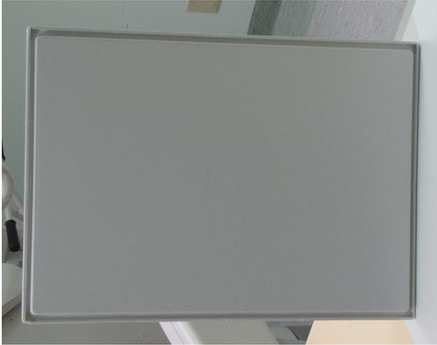
FIG. 15.2. Picture of a  $^{57}\text{Co}$  flood source.
