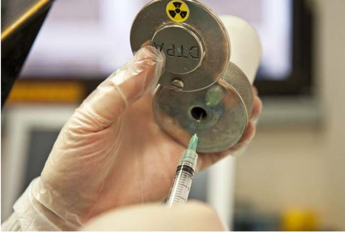
*FIG. 9.10. Shielded vial used to hold reconstituted radiopharmaceuticals.*
