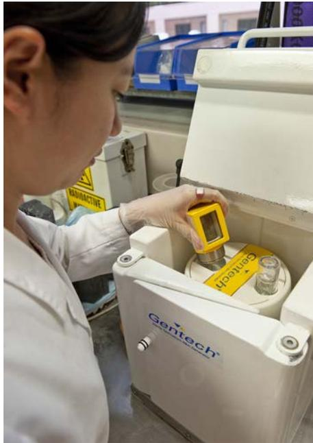
FIG. 9.9. Lead garage surrounding a  $^{99}\text{Mo}/^{99\text{m}}\text{Tc}$  generator:
