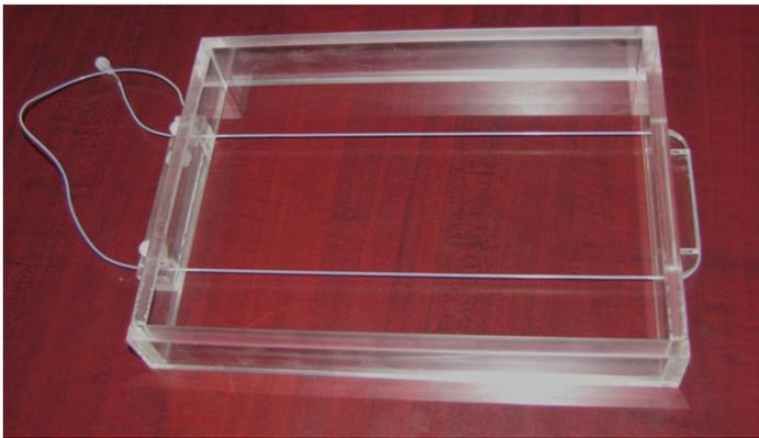
FIG. 15.6. Dual-line phantom for whole body resolution tests.
