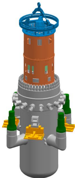
Fig.4. Reactor with other main equipment connected
