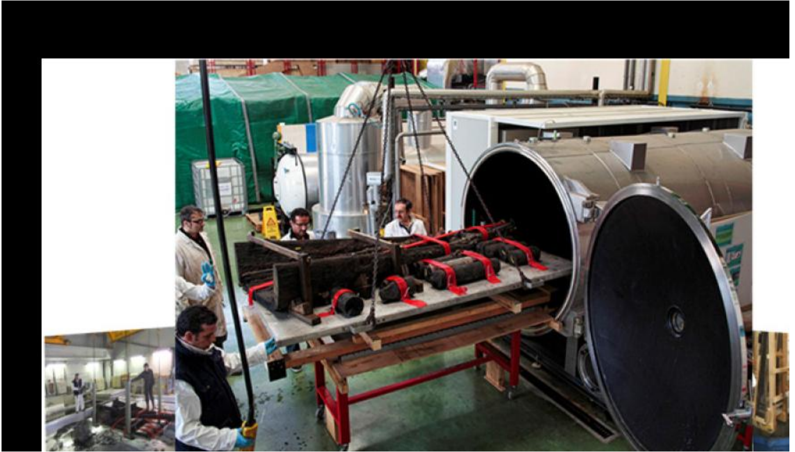
Freeze-drying after PEG impregnation
