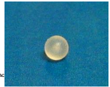
Co-60, Sc 46 particle in polypropylene ball, tracking liquid
