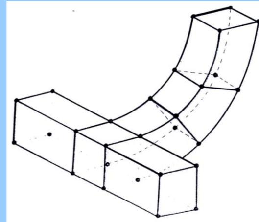
The blocks can have **curved edges**, to fit the problem geometry, but must remain topologically equivalent to a rectangular block
