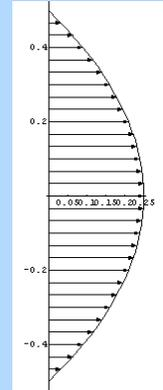
In the case of heat transfer due to a constant heat flux applied to the external surface, the temperature profile is quartic:
