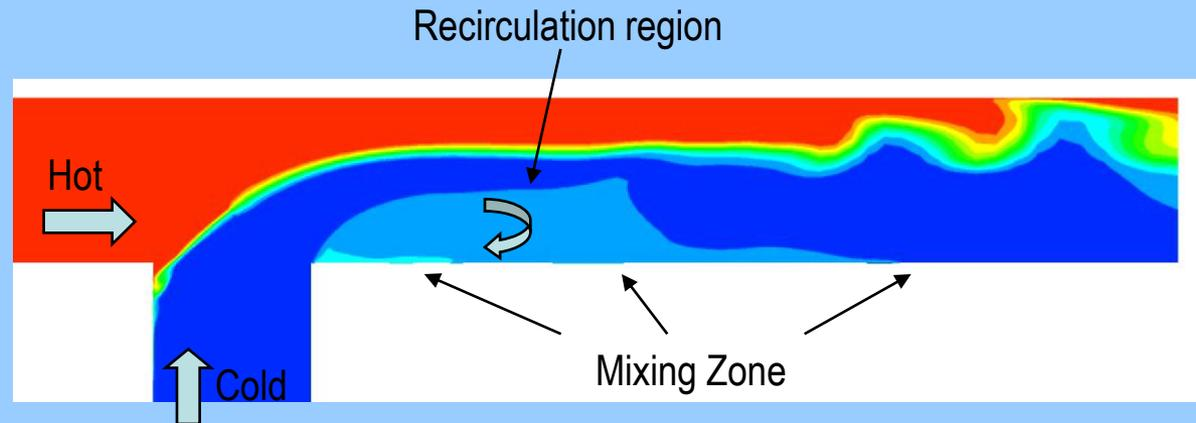
Most damaging thermal loads appear to be due to large-scale turbulent fluctuations; i.e. identification and quantification of non-steady phenomena of low frequency (1-10 Hz) are important.
