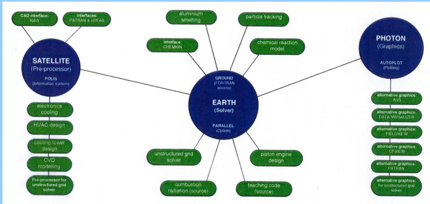
**Modular design:** central solver, pre-processor (mesh generator), post-processor (graphical display of results) and modules to link in, as needed for the particular application.
