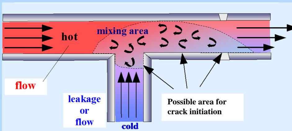
Can also occur as a result of thermal striping caused by alternate hot/cold jets.
