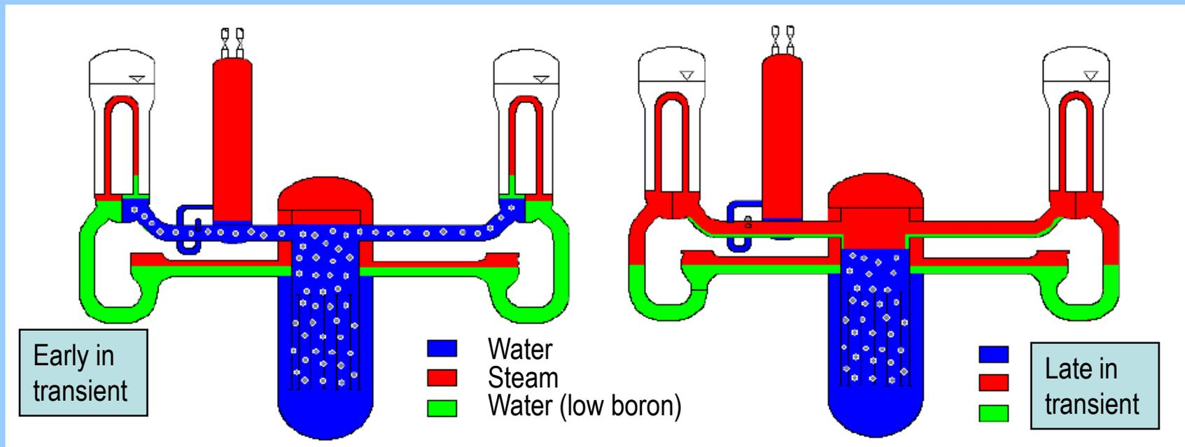
The dilution event occurs when natural circulation is re-established or a reactor coolant pump (RCP) is restarted. The low-borated water, if it remains unmixed, could be transported to the core and produce a power excursion.
