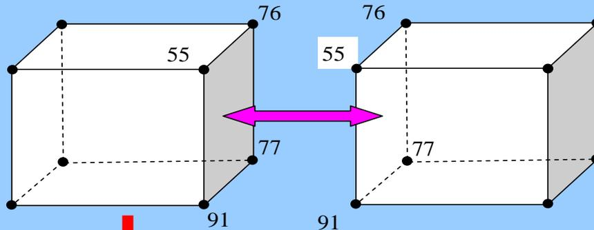
The **joining** of the E and W faces of adjacent (hexahedral) blocks is accomplished using the concept of **shared nodes**; i.e. nodes have the same number in the global node numbering system.
