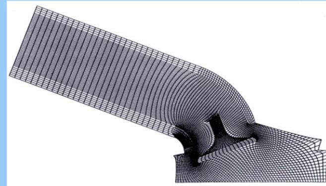
CFD is widely used in the aerospace and automotive industries. The concept of **moving meshes**, for example to represent the motion of engine exhaust valves, has been introduced. As the valve moves, the meshes in the vicinity are adapted to the new flow geometry.
