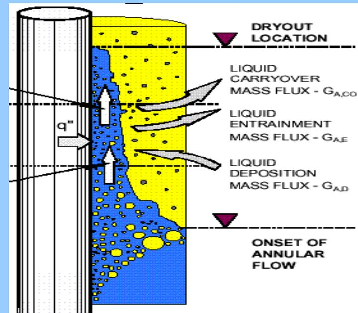
Can track liquid film using CFD
