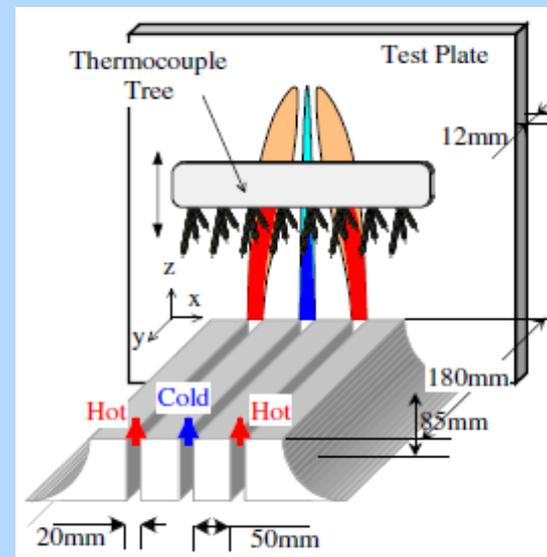
Thermal striping experiment at O-arai Engineering Center, Japan
