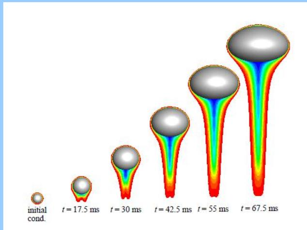
...are developed into multi-bubble configurations for the testing of bubble break-up and coalescence.
